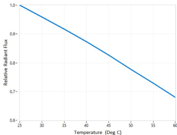
Figure 5. Relative radiant flux vs temperature
