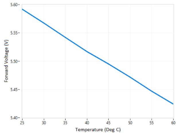
Figure 8. Forward voltage vs temperature
