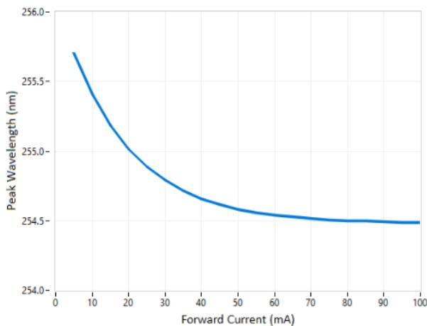
Figure 3. Peak wavelength vs forward current
