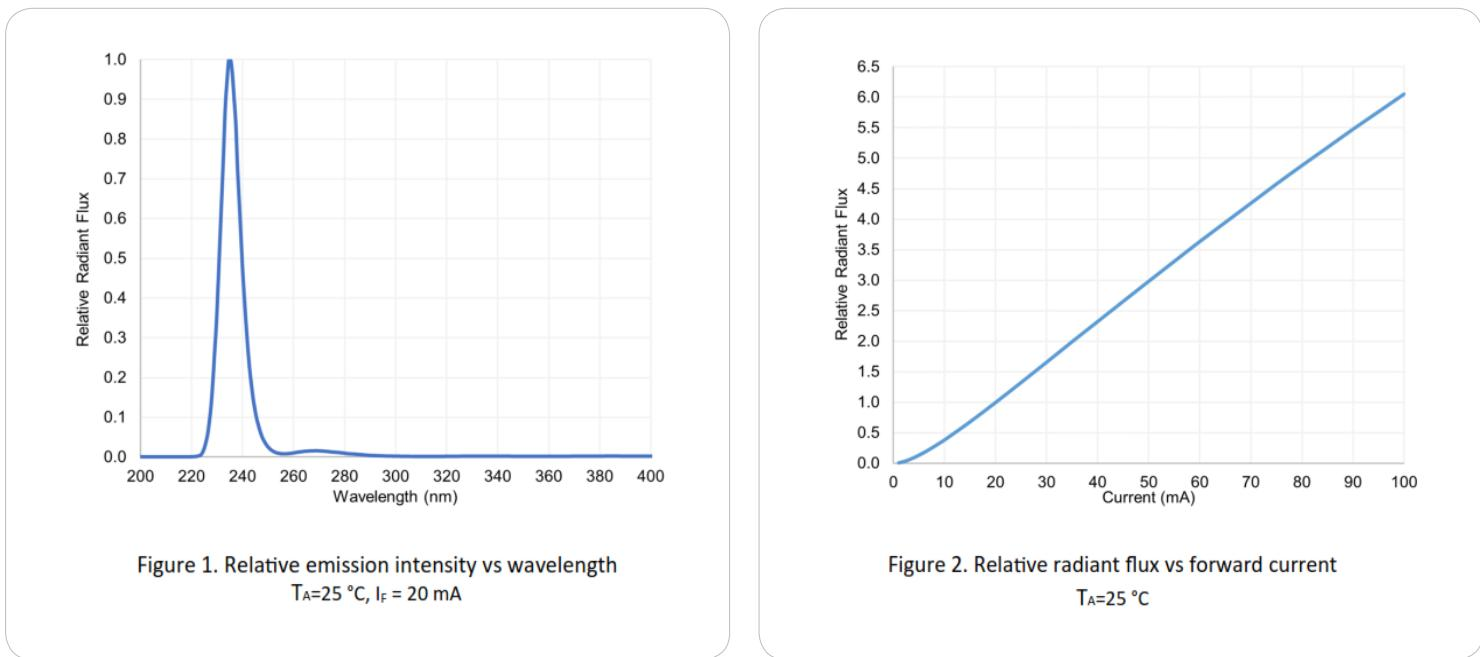
Figure 1. Relative emission intensity vs wavelength
