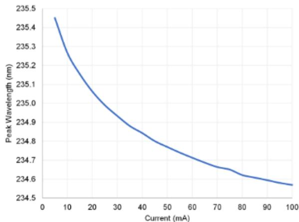
Figure 3. Peak wavelength vs forward current
