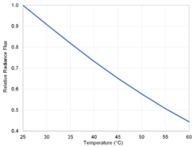
Figure 5. Relative radiant flux vs temperature
