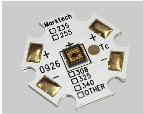
Aluminum Core Board 0.040" (1.02mm) Thickness
