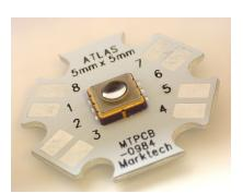
Aluminum Core Board 0.040" (1.02mm) Thickness Overall Board Dimensions: +/- 0.010" (0.254mm)
