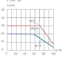
MAXIMUM FORWARD DC CURRENT VS, AMBIENT POINT TEMPERATURE.
